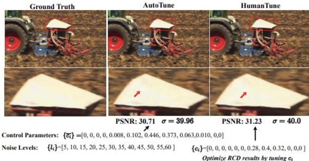
Figure 5. Example of RCD denoising results by AutoTune and HumanTune on Set8. AutoTune module provides reference control parameters, *i.e.*,  $\{\bar{c}_i\}_{i=1}^L$ , to generate the denoising result, and it can be further improved by fine-grained artificial tuning (HumanTune), *i.e.*,  $\{c_i\}$ , without changing the noise intensity (both  $\sigma = 40$ ).
