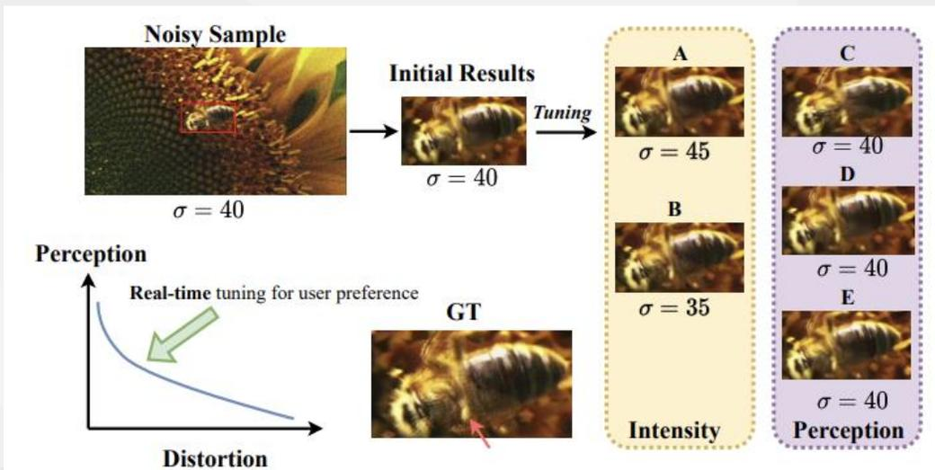
Figure 1. Real-time controllable denoising allows users further tuning the restored results to achieve Perception-Distortion trade-off. **A-B**: tuning with changing denoising intensity. **C-E**: tuning without changing denoising intensity.
