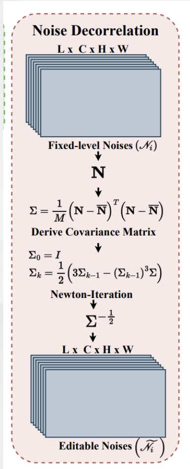
Transform fixed-level noises to editable noises by batch whitening
