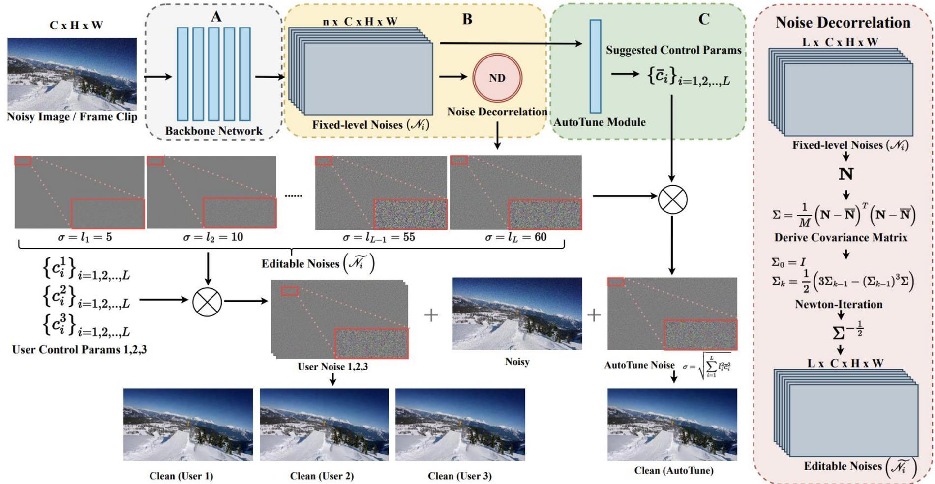
Figure 3. Pipeline overview of proposed RCD framework. **A:** Backbone network for generating multi-level noise maps. **B:** Noise Decorrelation module for editable noises. **C:** AutoTune module for providing reference control parameters for users.
