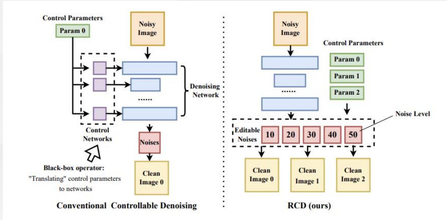
In this work, We propose Real-time Controllable Denoising method (RCD), a lightweight pipeline for enabling rapid denoising control to achieve Perception Distortion Balance.
