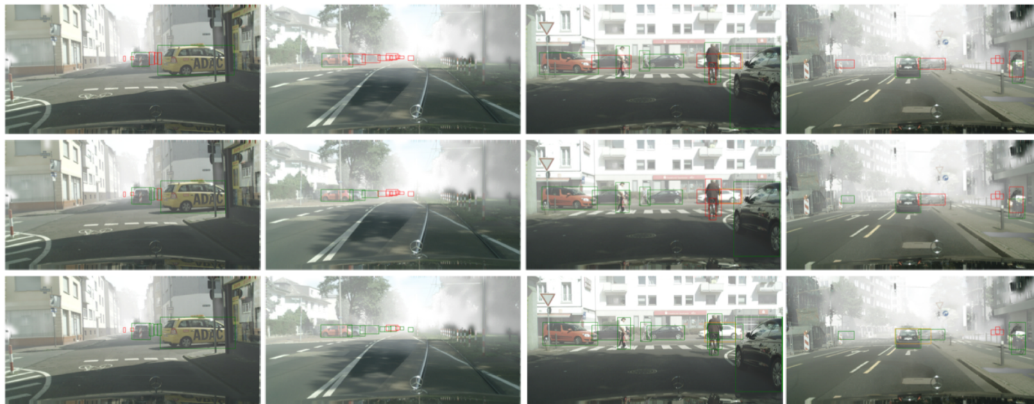
Figure 5. Qualitative results on the target domain of Cityscapes to Foggy Cityscapes for Source Only [36] (top row), SIGMA [19] (middle row) and Ours (bottom row). Green , red and orange boxes indicate true positive (TP), false negative (FN) and false positive (FP), respectively. We set the score threshold to 0.7 for better visualization. Best appreciated when viewed in color and zoomed up.
