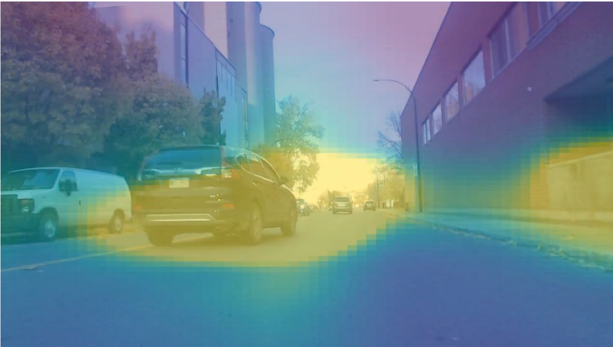
Beamformed Sound Pressure Signal Overlaid on Traffic Video
